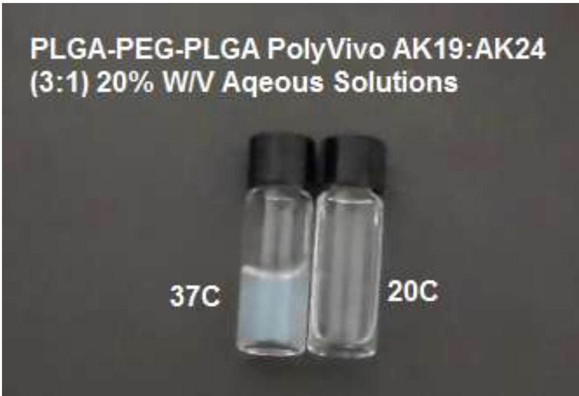
Figure 8. Results of tube tip test 3:1 AK19:AK24 solution at 37°C (left) and 20°C (right) respectively. Note solution flows easily at 20° C but is a gel at 37° C.
