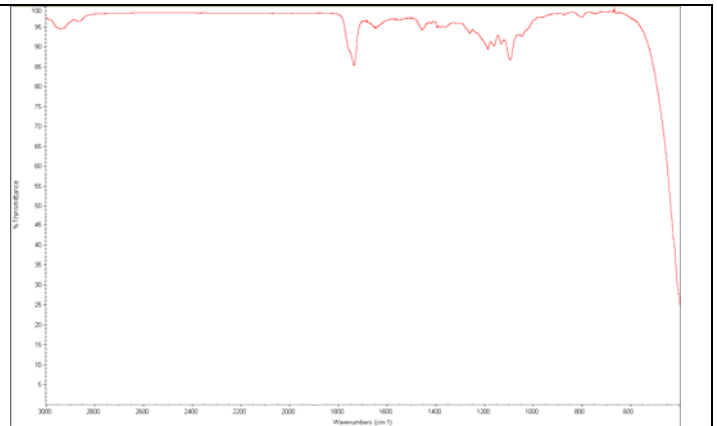
FTIR Analysis: Collected from cast-film on KBr salt-plate placed in Protégé 460 Spectrometer (Nicolet) and analyzed in Transmission E.S.P. mode.
