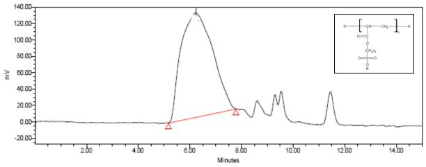
Analysis Method (as provided by supplier): Agilent 1050 Series with 1 ml/min 0.1N sodium nitrate in HPLC water flow across PL aquagel Mixed-OH columns. Detection via Differential Refractive Index (128x, 40°C), calibrated against EasiVial® poylethylene glycol/oxide standards.
