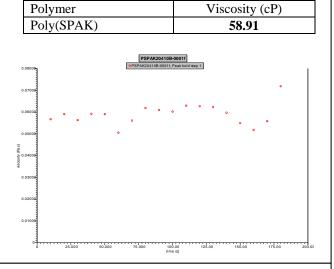
Analysis Method: 1% solution in distilled water placed in AR550 rheometer with 2° 60mm plate temperature held at 25C rotated at 60RPM 6 measurements made every 10 seconds over the course of 1 minute.
