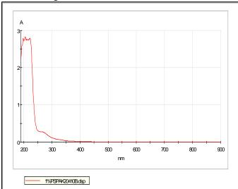
Analysis Method: 1% solution in distilled water measured on Genesys-6 against a distilled water blank. Spectrum recorded at 1nm resolution from 900-190nm wavelength using visionlite software.
