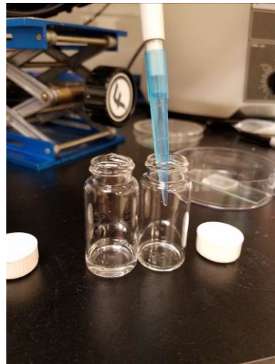
D. Transfer of 1 mL 5% AI147 into vial containing dissolved Irgacure 2959
